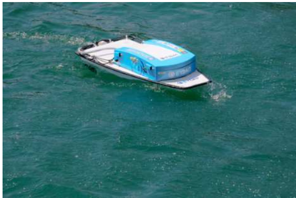
Unmanned Surface Vehicles for testing water (INTCATCH)
